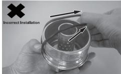
○ Do not pull and apply extra tension to the O-ring
